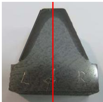
Qualified induction hardening and teeth grinding
